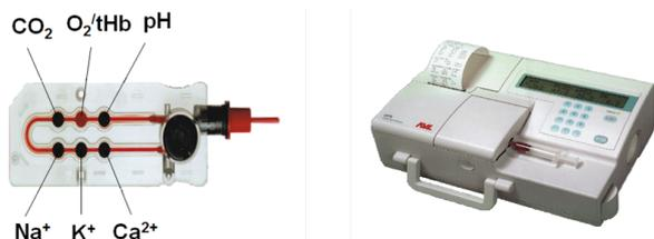
Figure 4: A disposable cassette (left) and OPTI critical care analyser (right). The black spots (left picture) are organic polymer fibre mats attached to the appropriate sensor molecules for:  $Na^+$ ,  $K^+$ ,  $Ca^{2+}$ ,  $pH$  and  $CO_2$ . The orange spot is the sensor for  $O_2$ . Adapted from reference 20 and reproduced with permission of the Royal Society of Chemistry (RSC).
